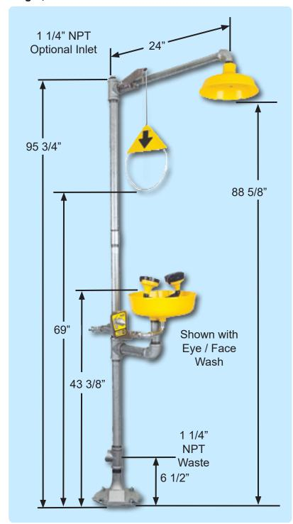
• VALVES: Chrome plated bronze stay open ball valves with chrome plated balls, stainless steel valve stems, stainless steel push plate with actuation graphic (eye/face wash) and stainless steel pull rod assembly with actuation graphic (shower). Valve Size 1", eye face wash 1/2" Strainer Tee option: 1/2" BCP, 16 mesh.
